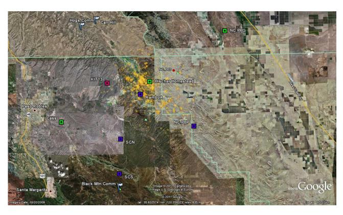
Figure 2.33: Planned locations for TremorScope stations. Gold stars: Tremor locations. Colored squares: TremorScope sites. NC.PBP and NC.PPG are currently operated by the USGS Menlo Park and have short period vertical geophones and analog telemetry. Sites Cass, SCS, NC.PBP and NC.PPG will be borehole stations. SCN and SCS are collocated with PBO GPS stations. Telemetry will go via radio to Carr Hill, Hogs Canyon Comm. or Black Mountain Comm.
