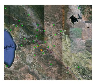
Figure 2.34: Location map of San Juan Bautista segment of the San Andreas fault. Purple circles are USGS and Univ. Colorado, Boulder creepmeters; green circles are PBO and BARD continuous GPS stations. Orange circles are the locations of M3 and higher earthquakes in January, 2011, which are assumed to have occurred on a southwest dipping San Andreas fault.
