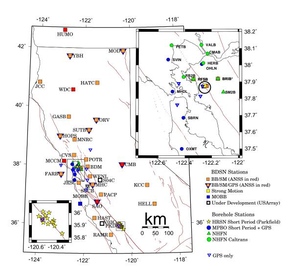
Figure 3.1: Map illustrating the distribution of BSL networks in Northern and Central California. UCGS and CalEMA contribute to operating these stations. ANSS backbone stations are shown in red. In the inset map, the shown stations in the circle include BRK, BKS, CMSB, VAK, BL88, and BL67. \* Station BRIB is also a GPS and mPBO site. Abbreviations: BB/SM - Broadband/Strong Motion; BB/SM/GPS - Broadband/Strong Motion/GPS
