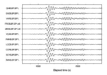
Figure 3.18: Plot of surface wave seismograms of the teleseismic  $M_w$  9.0 earthquake near the east coast of Honshu, Japan (Lat.: 38.322N; Lon.: 142.69E; depth 32 km) occurring on March 11, 2011 05:46:23 (UTC) recorded on the BP1/SP1 (vertical) channels of the 11 HRSN borehole stations in operation at the time. Here, vertical component geophone (velocity) data have been 0.02-0.05 Hz bandpass filtered and normalized by the maximum amplitude for each trace.
