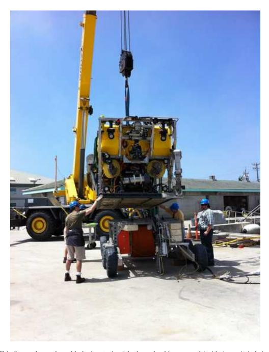
Figure 3.7: This figure shows the cable laying tool, with the red cable wrapped inside it, as it is being mounted on the bottom of the ROV Ventana prior to installation. The sharp metal "edge" hanging from the middle of the sled was used to dig a narrow trench in the seafloor as the cable was laid down, so as to bury it and protect it from trawling,. Courtesy of Paul McGill, MBARI.
