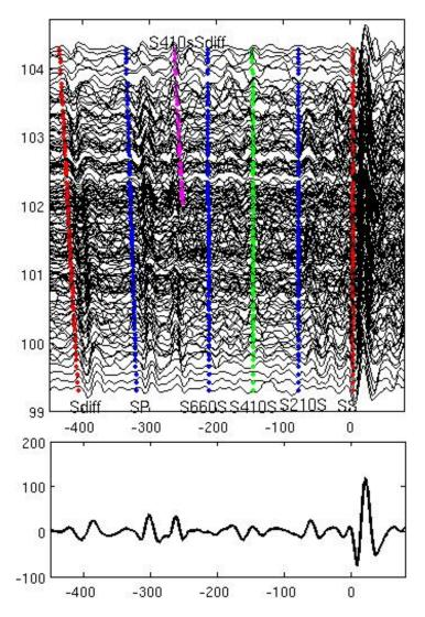
Figure 2.61: Top: Seismic profile of SS precursors with predicted traveltime of the IASP91. Bottom: Stacked data using the SS phase as a reference.
