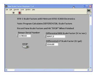
Figure 3.35: Example snapshot of the Metrozet Scale Factor Applet V1.20 results screen showing the serial number and correponding differential BRB and LP scale factors for use with the E300 electronics.
