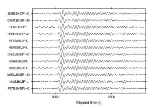
Figure 3.16: Plot of surface wave seismograms of the teleseismic  $M_w$  9.0 earthquake near the east coast of Honshu, Japan (Lat.: 38.322N; Lon.: 142.369E; depth 32 km) occurring on March 11, 2011 at 05:46:23 (UTC) recorded on the DP1/EP1 (vertical) channels of the 12 NHFN and mPBO borehole stations in operation at the time. Here, vertical component geophone (velocity) data have been 0.02-0.05 Hz bandpass filtered and normalized by their maximum amplitudes.
