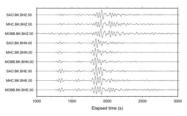
Figure 3.8: This figure shows MOBB broadband data along with traces from SAO and MHC for the M7.0 earthquake off the east coast of Honshu, Japan  $(2011/07/10~00:57:12~\mathrm{UTC})$ . A 0.01-0.03 Hz BP filter was applied. They are in ground velocity and are normalized by their maximum amplitudes.
