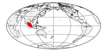
Figure 2.64: SS ray path from a shallow event ( $m_b$  6.7; depth 38 km) to a station (T28A) in the US Transportable Array. The location of the bounce point is denoted by a cross.
