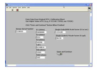
Figure 3.34: Example snapshot of the Metrozet Scale Factor Applet V1.20 input showing the serial number and component values.
