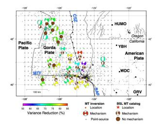
Figure 2.43: Map of the Mendocino Triple Junction region showing the grid of point sources (crosses), the four seismic stations (HUMO, ORV, WDC and YBH), the regional seismicity since 1990 (black dots), and the studied events that are shown in brown for the catalog solutions and are color-coded by the VR for the inversion solutions.
