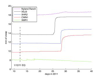
Figure 2.35: Creepmeter records from 1/9/2011 - 2/9/2011 for one U. Colorado (NYR) and four USGS creepmeters on the San Andreas fault. A small offset is seen at the time of the earthquake, likely due to shaking of the instrument during the event, rather than fault slip. A creep event occurs at SAOB 13 days after the M4.1 earthquake; after 4 more days, a creep event occurs at XHR2 and CWN1.
