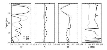
Figure 2.71: First order harmonic decomposition of receiver function amplitude as a function of inferred depth (Equation 2.2). Results for  $S_V$  and  $S_H$  are shown in black and grey, respectively.  $R^2$  shows the fit to Equation (2.2). The A component represents a constant amplitude term. B and C are amplitude and phase of a fitted cosine term.
