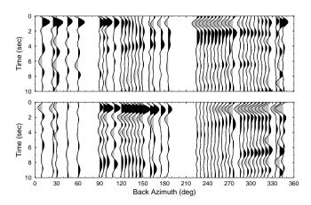
Figure 2.70: Receiver functions from station SAO near San Juan Bautista, Northern California.  $S_V$  (top) and  $S_H$  (bottom) components sorted by back-azimuth of incoming wavefield. Black is positive and grey is negative.
