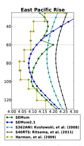
Figure 2.50: Comparison of  $V_S$  profiles at an arbitrary point beneath the EPR. Dotted lines at 30 and 60 km indicate Moho depth in the old and new crustal models. (Mean of *Harmon*, et al. (2009) regional  $V_{SV}$  model shown)
