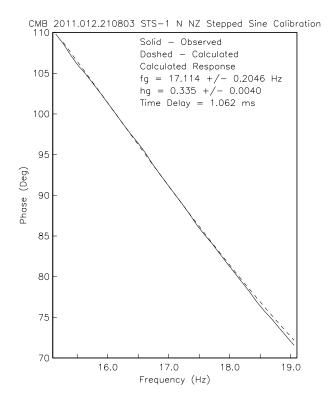
Figure 3.33: CMB STS-1/E300 North Component High-Frequency Response. The plot shows the observed (solid line) and calculated (dashed line) response to the stepped-sine stimuli. The least-squares solution is  $f_g{=}17.114{\pm}0.2046{\rm Hz}$  and  $h_g{=}0.335{\pm}0.0040$ . There is an internal time delay of 1.062 msec between the stimuli applied to the calibration coil and stimuli recorded by the data logger, which is accounted for in the algorithm.
