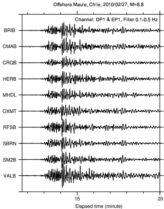
Figure 3.15: Plot of P-wave seismograms of the teleseismic  $M_w$  8.8 earthquake in the offshore Maule, Chile (Lat.: 35.909S; Lon.: 72.733W; Depth: 35 km) occurring on February 27, 2010 at 03:34:14 (UTC), recorded on the DP1 (vertical) channels of the 10 NHFN borehole stations in operation at the time. Here, vertical component geophone (velocity) data have been 0.1-0.5 Hz bandpass filtered.
