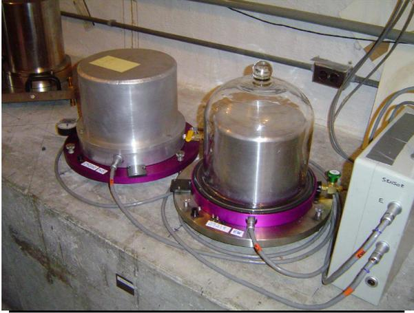
Figure 3.31: STS-1 seismometers in the Byerly Vault installed in a new pressure vessel (left) and on a warplless baseplate with a glass bell (right).
