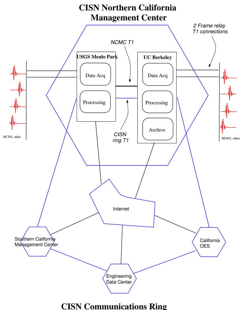
Figure 3.11: Schematic diagram illustrating the connectivity between the real-time processing systems at the USGS Menlo Park and UC Berkeley, forming the Northern California Management Center, and with other elements of the CISN.
