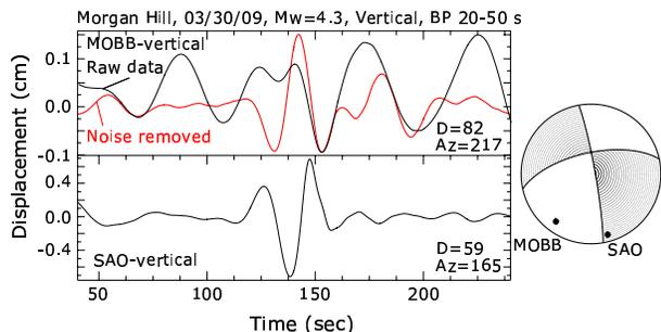
Figure 3.8: Comparison of raw and filtered traces on the vertical component at MOBB, before and after deconvolution with the DPG data to remove infragravity wave related noise, for the Morgan Hill  $M_w$  4.3 earthquake of 03/30/09. The bottom trace shows the corresponding record at land station SAO. On the right is shown the earthquake mechanism with the azimuths of the two stations.
