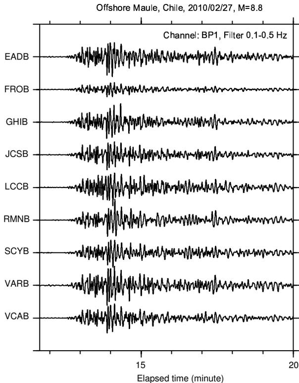
Figure 3.17: Plot of P-wave seismograms of the teleseismic  $M_w$  8.8 earthquake in the offshore Maule, Chile (Lat.: 35.909S; Lon.: 72.733W; Depth: 35 km) occurring on February 27, 2010 03:34:14 (UTC) recorded on the DP1 (vertical) channels of the 9 HRSN borehole stations in operation at the time. Here, vertical component geophone (velocity) data have been 0.1-0.5 Hz bandpass filtered.
