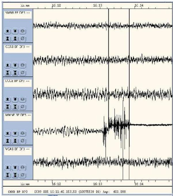
Failure of MMNB (4th waveform from top) between 16:13 and 16:14 (11:13 and 11:14 local time) on Aug 13, 2009 (Same day as clean-up effort). At this time background noise transitions to instrumental noise only.
