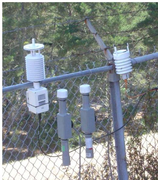
Figure 3.26: Cluster of MET sensors under test at BRIB. The sensors from left to right are; Paroscientific; BSL MET 2, BSL MET 1, and Vaisala. The electronics for the BSL MET sensors are remotely located approximately 40 feet away in the vault which contains the BRIB supporting hardware.
