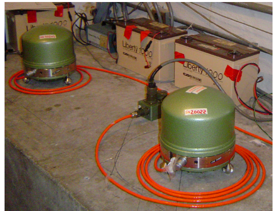
Figure 8.4: Photo of STS-2 sensors #50205 (right) and #20022 (left) after they were installed and leveled on the seismic pier in the BKS vault. After this photo was taken, the sensors were covered with a couple layers of R-13 fiberglass batt insulation to minimize temperature variations and improve their low frequency performance.
