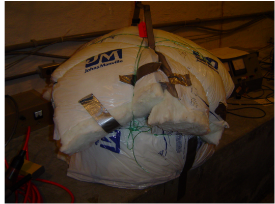
Figure 8.9: Photo of fiberglass batt insulation surrounding the pressure sphere.
