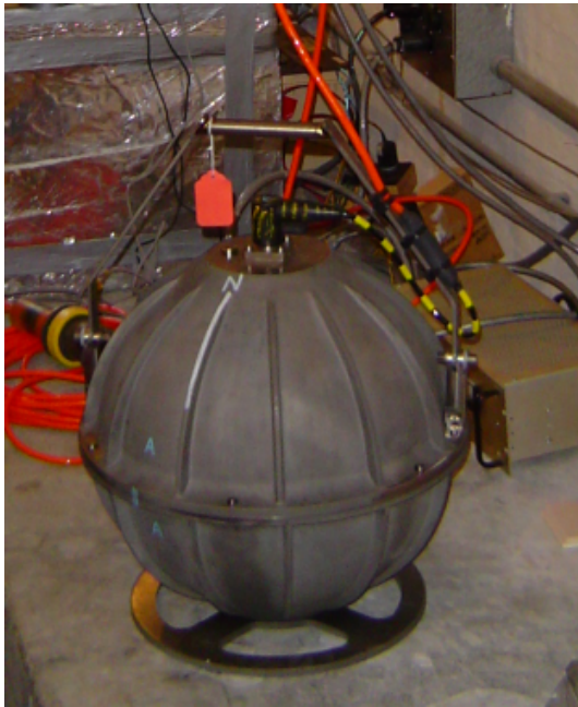
Figure 8.8: Photo of cast titanium pressure sphere housing Keck OBS #T1046. The disc shaped base is standing on three ceramic washers for stability on the seismic pier. The orange signal cable exiting at the top of the sphere is draped overhead to minimize the generation of noise at the cable responds to temperature changes.
