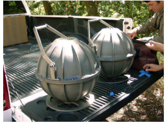
Figure 9.5: Custom made titanium pressure spheres which are designed for deployment at depths of up to 3.5 km. The hemispheres were made using an injection molding process. There are two access ports drilled into the flat top of each sphere, one for the penetrator containing the wiring cable and one for purging with argon gas (and for relieving any pressure differences so that the hemispheres can be separated). The handle on top is designed for the Remote Operated Vehicle (ROV) which deploys the sphere on the sea floor.
