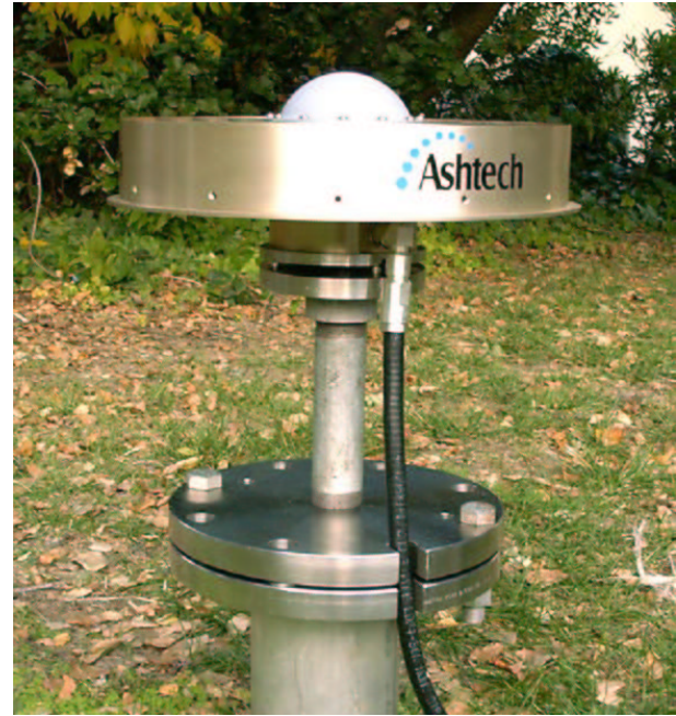
Figure 8.5: GPS antenna mount. The bottom flange is welded to the top of the borehole casing. The upper flange can be removed and replaced with sub-0.1 mm repeatability to provide access to the interior of the casing.
