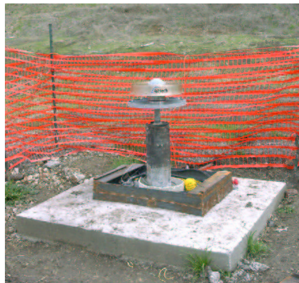
Figure 9.5: GPS antenna mounted on top of casing at OHLN. The final installation includes a SCIGN antenna dome and a steel protective shroud that envelopes the casing.
