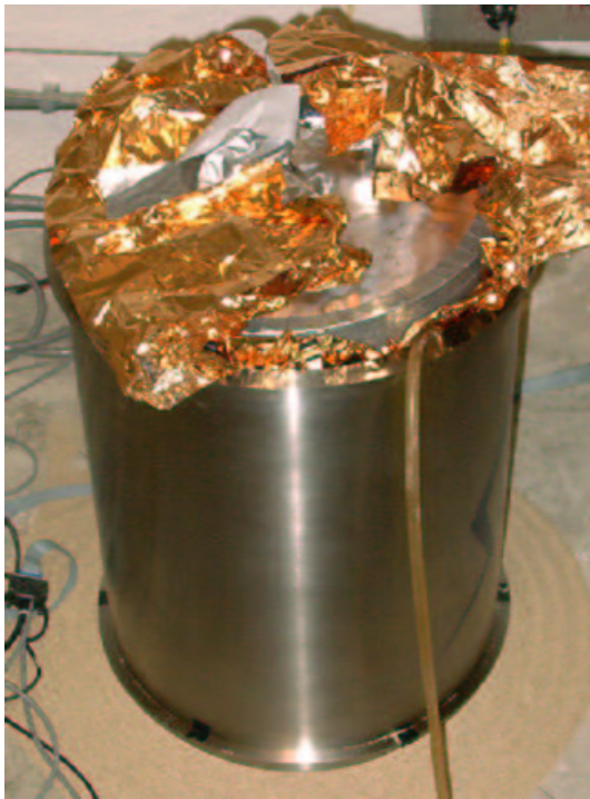
Figure 11.12: Photo of the space blanket insulation and the space filling urethane foam space filling plug in the titanium pressure vessel with the titanium end cap removed.
