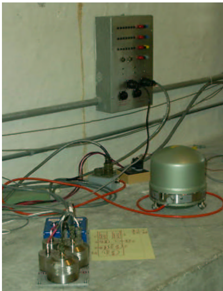
Figure 11.5: Interconnecting patch panel (top center) which routes the signals from the sensors under test (lower left and STS-2 reference sensor center right) to the Q4120 data logger.
