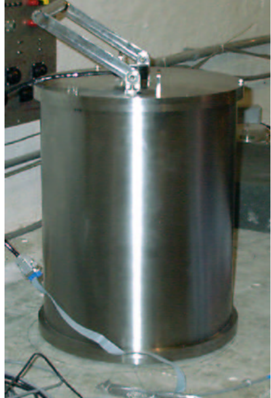
Figure 11.11: Photo of the titanium pressure vessel resting on a \sim 1 cm thick bed of kiln dried fine sand on the concrete pier.
