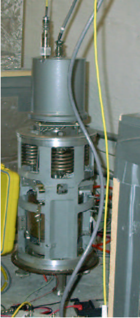
Figure 11.6: Simple vertical shake table, constructed using a Johnson-Matheson Model 6840 short-period seismometer, with a PMD sensor mounted on top of the shake table for testing.
