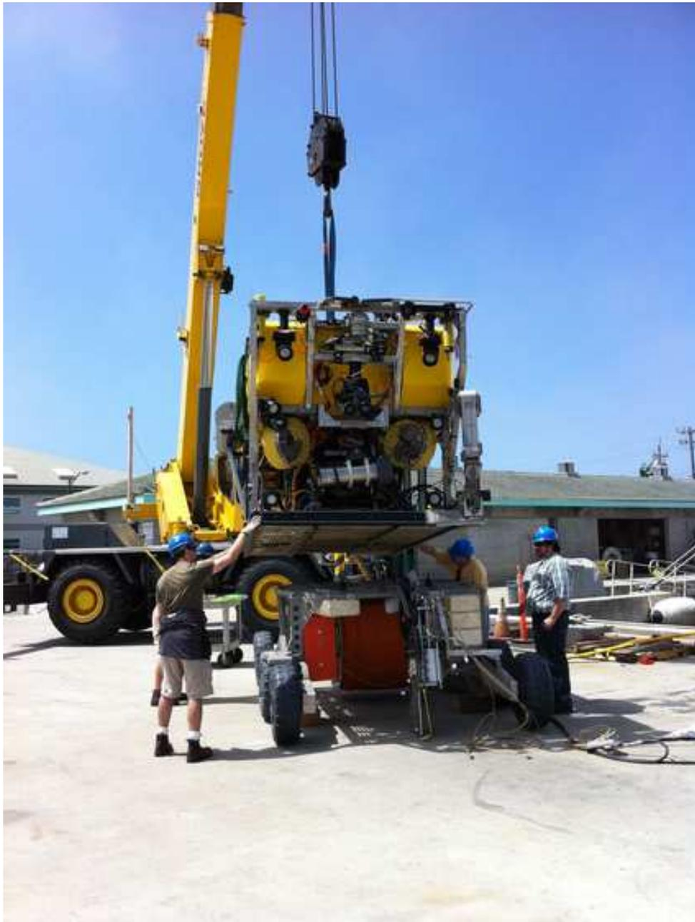
Figure 3.7: This figure shows the cable laying tool, with the red cable wrapped inside it, as it is being mounted on the bottom of the ROV Ventana prior to installation. The sharp metal "edge" hanging from the middle of the sled was used to dig a narrow trench in the seafloor as the cable was laid down, so as to bury it and protect it from trawling,. Courtesy of Paul McGill, MBARI.
