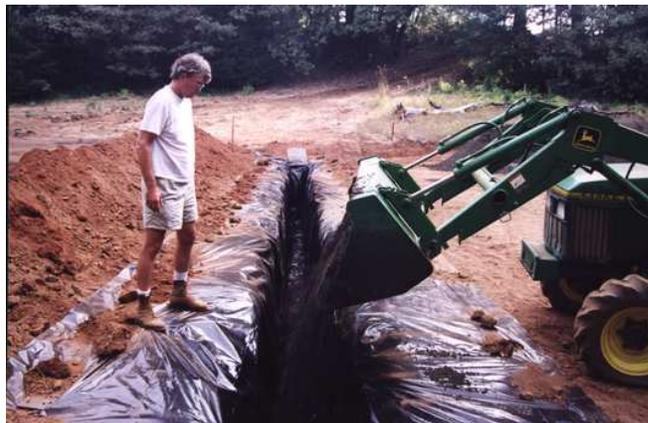
**Figure 7:** Data acquisition prior to construction of second trench, using “fan” geometry. Source point in this photo is one meter from one side of the trench, and receiver line is one meter from the opposite side of the trench. Shooter is standing in the trench, with PVC piezometers on either side of him that are used to measure water table in trench.
