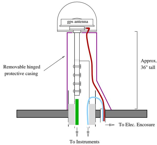
Figure 4: Design of the Mini-PBO GPS antenna mount on top of casing.
