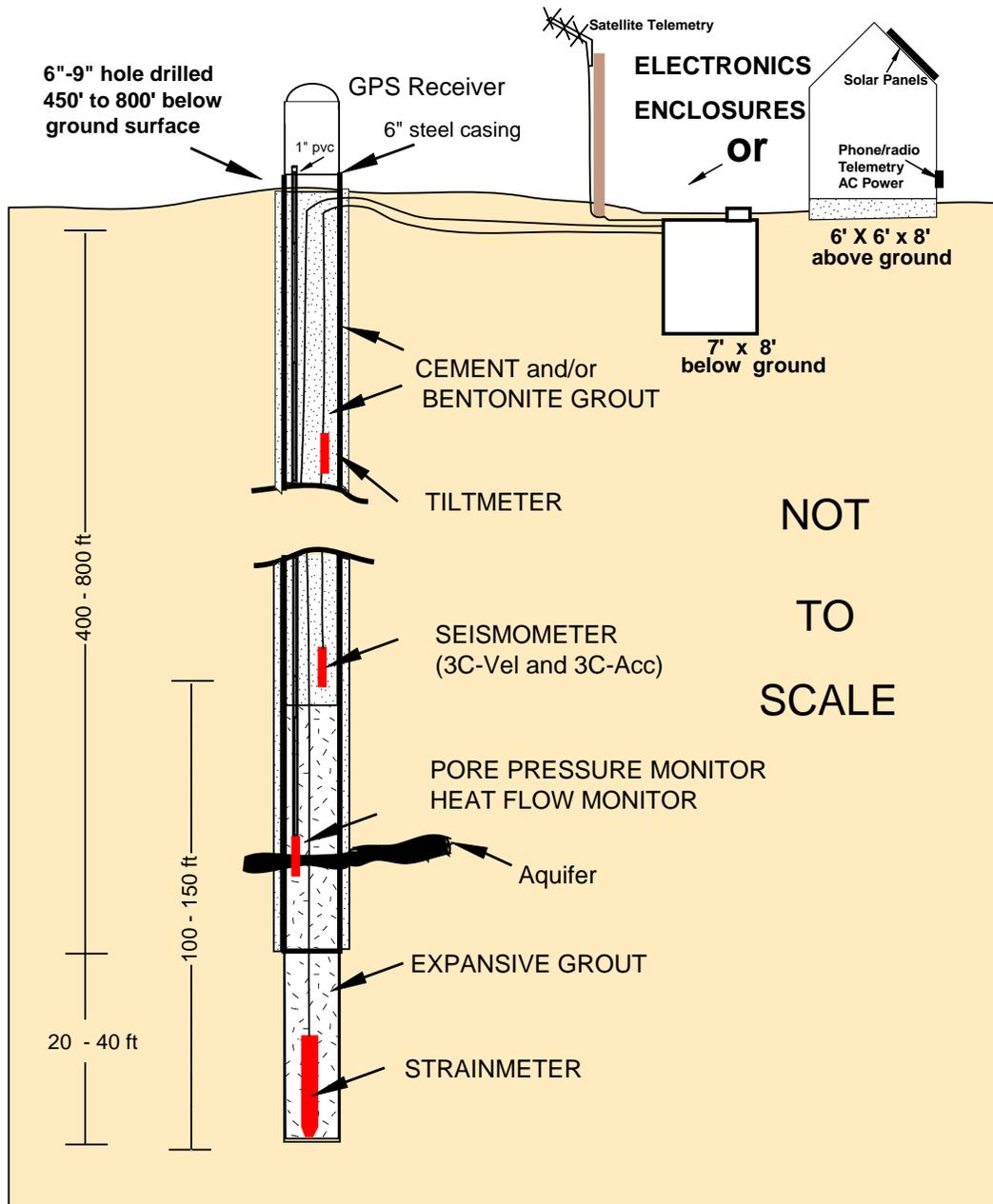
Figure 3: Design of the Mini-PBO borehole installation, showing the emplacement of the instruments downhole and the GPS receiver on the top.
