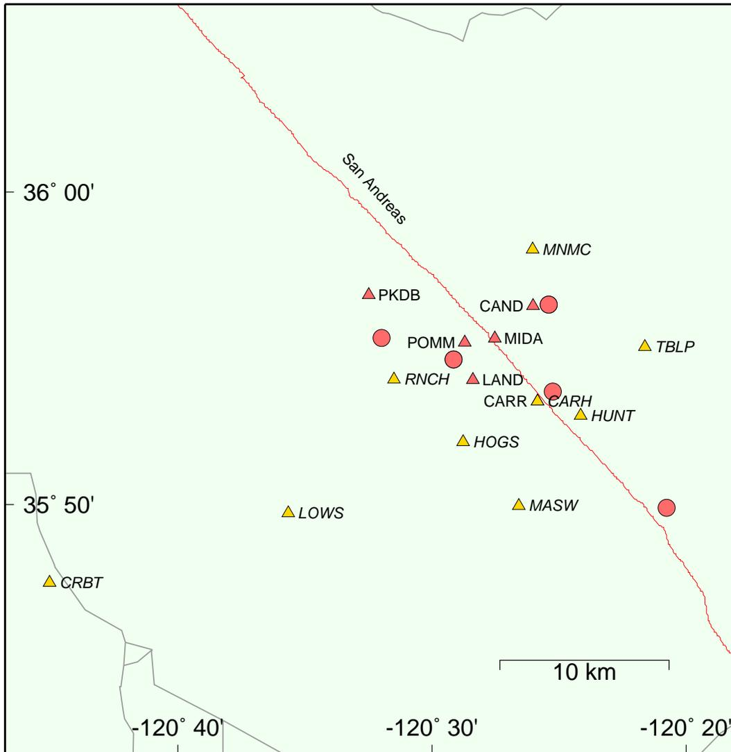
Figure 2: Location of the permanent GPS sites installed near Parkfield in the framework of this project (yellow triangles) along with other relevant instruments (red triangles:GPS; red circles: borehole strainmeters).
