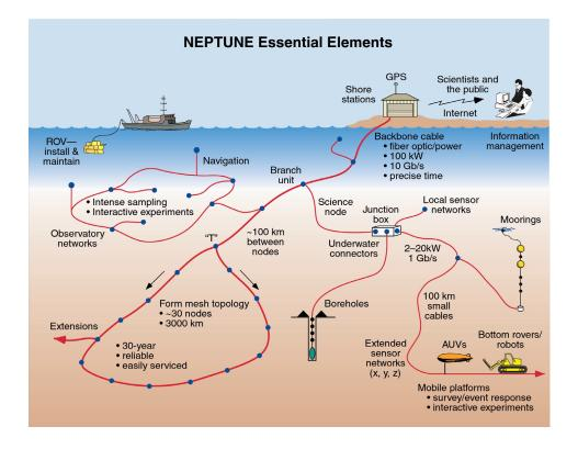
Figure 2. Land-based scientists and the public are linked in real time and interactively with sensors, sensor networks, and various mobile sensor platforms in, on, and above the seafloor. NEPTUNE's fiber-optic/power cable and associated technology provide the enabling network infrastructure.
