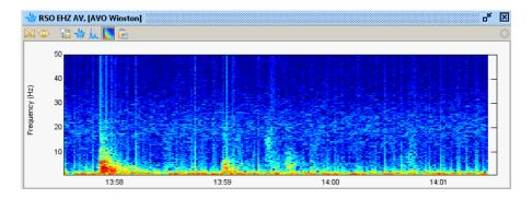
Figure 11: A typical Real-time Wave Viewer showing a just-occurred microquake
