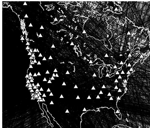
Figure 13.45: Data coverage - Paths of teleseismic events with  $M_w \geq 6$  recorded at North American stations (indicated by white triangles), for which high quality fundamental mode Rayleigh wave packets have been selected.
