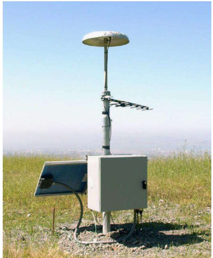
Figure 8.3: L1 system installation at GRIZ. This autonomous system uses solar panels (mounted in back) and Freewave radios (with Yagi antenna mounded on pole below GPS antenna). GPS receiver, radio, solar power regulators, and backup batteries are in the electronics box mounted in front.
