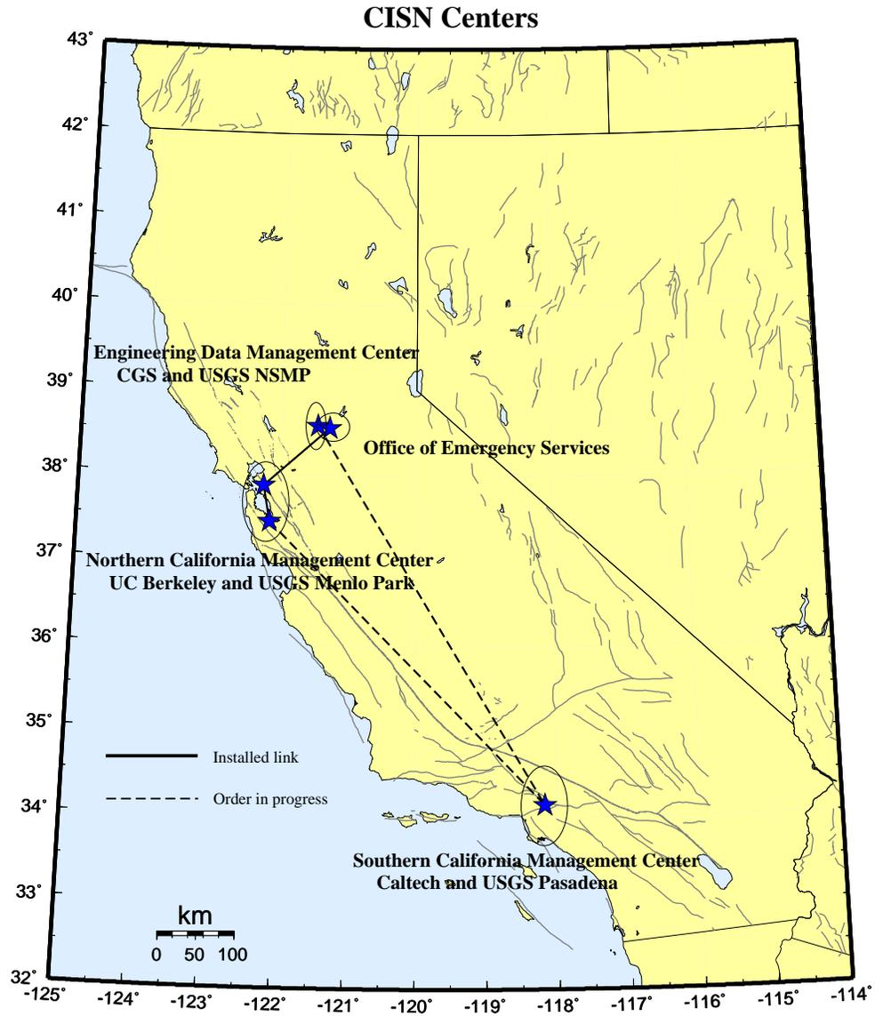
Figure 3.1: Map showing the geographical distribution of the CISN partners and centers. The communications "ring" is shown schematically with installed links (solid lines) and ordered links (dotted lines).
