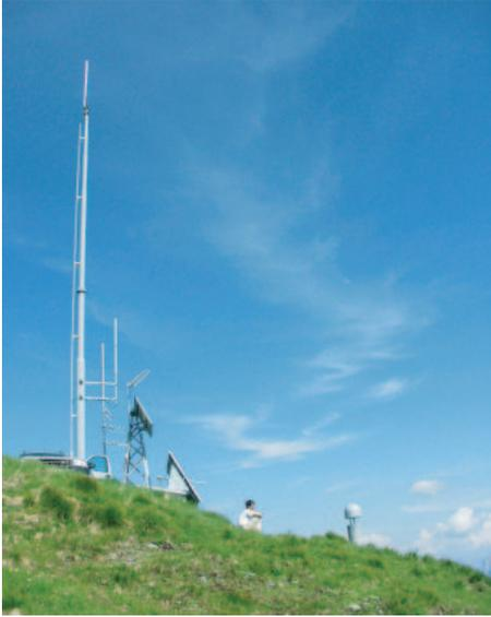
Figure 15.29: GPS station at Zouf Plan (ZOUF), collocated with seismic station ZOU. The 1-m high concrete pier with GPS antenna and dome mounted on top are on the right. Solar panels and radio antenna mast for the seismic station are on the left.
