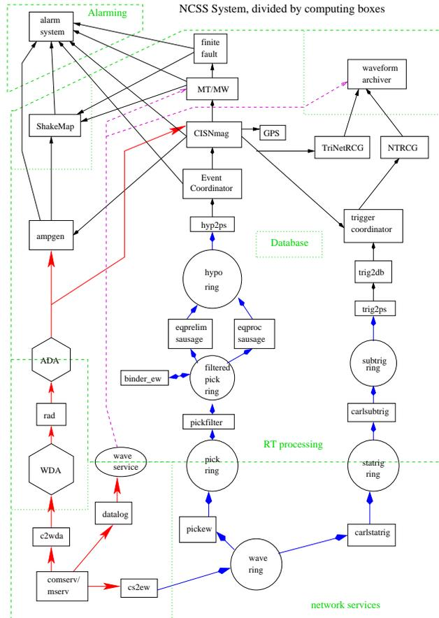
Figure 3.33: Schematic diagram of the planned NCSS system. The design combines elements of the Earthworm, TriNet, and REDI systems
