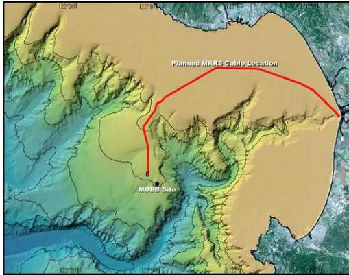
Figure 3.6: Location of the MOBB station in Monterey Bay, California, against seafloor and land topography. The path of the MARS cable is indicated by the solid line.
