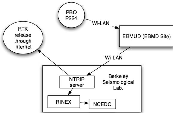
Figure 3.16: Present BSL operations at EBMD site and planned operations between the PBO site P224 and BSL. Since its installation in 2003, the EBMD site had been sending data to BSL using an internet DSL connection. The data collected (Trimble 5700 receiver) are now sent to BSL using a WI-LAN radio connection. The connection represents an upgrade of the quality of the radio link. The data collected here are thus more safely sent to BSL in case of a large seismic event.
