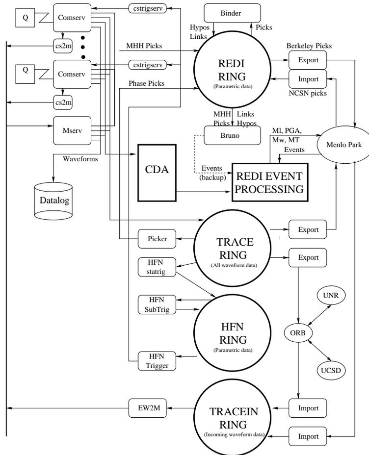
Figure 3.25: Dataflow in the REDI processing environment, showing waveform data coming in from the Quanterra data loggers (Q) into `comserv`. From `comserv`, data are logged to disk (via `datalog`), distributed to other computers (`mserv`), fed into the CDA for REDI processing, and spooled into a trace ring for export.
