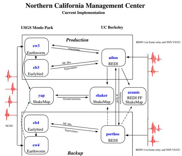
Figure 3.31: Detailed view of the current Northern California processing system, showing the two Earthworm-Earlybird-REDI systems, the two ShakeMap systems, and the finite-fault system.
