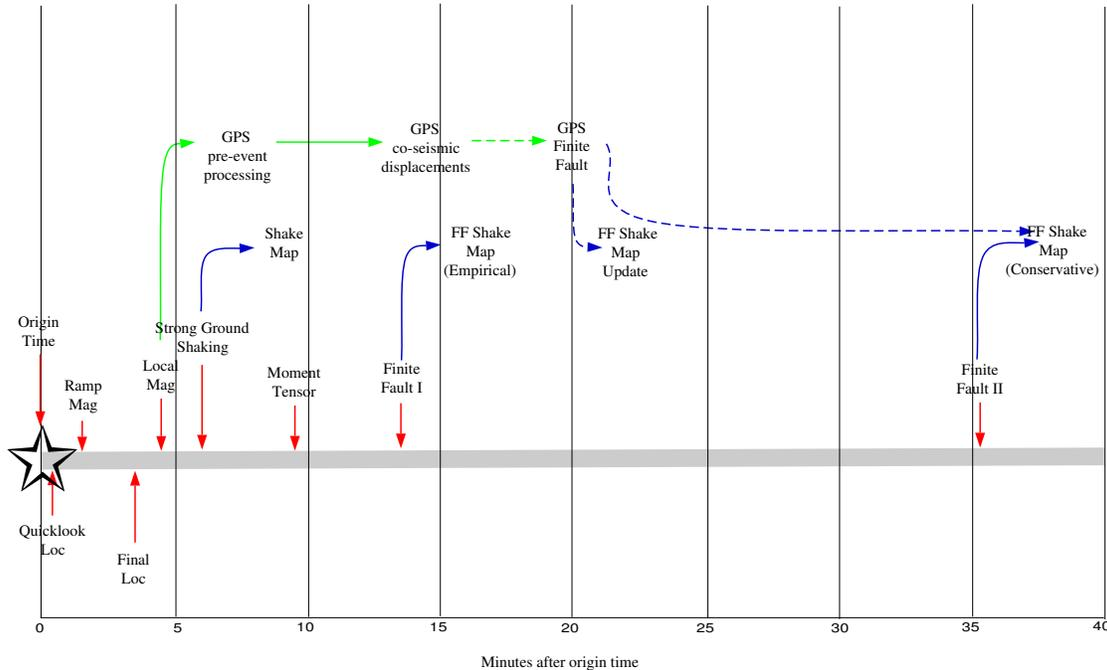
Figure 3.32: Illustration of the current (solid lines) and planned/proposed (dotted lines) development of real-time processing in northern California. The Finite Fault I and II are fully implemented within the REDI system at UC Berkeley and are integrated with ShakeMap. The resulting maps are still being evaluated and are not currently available to the public.
