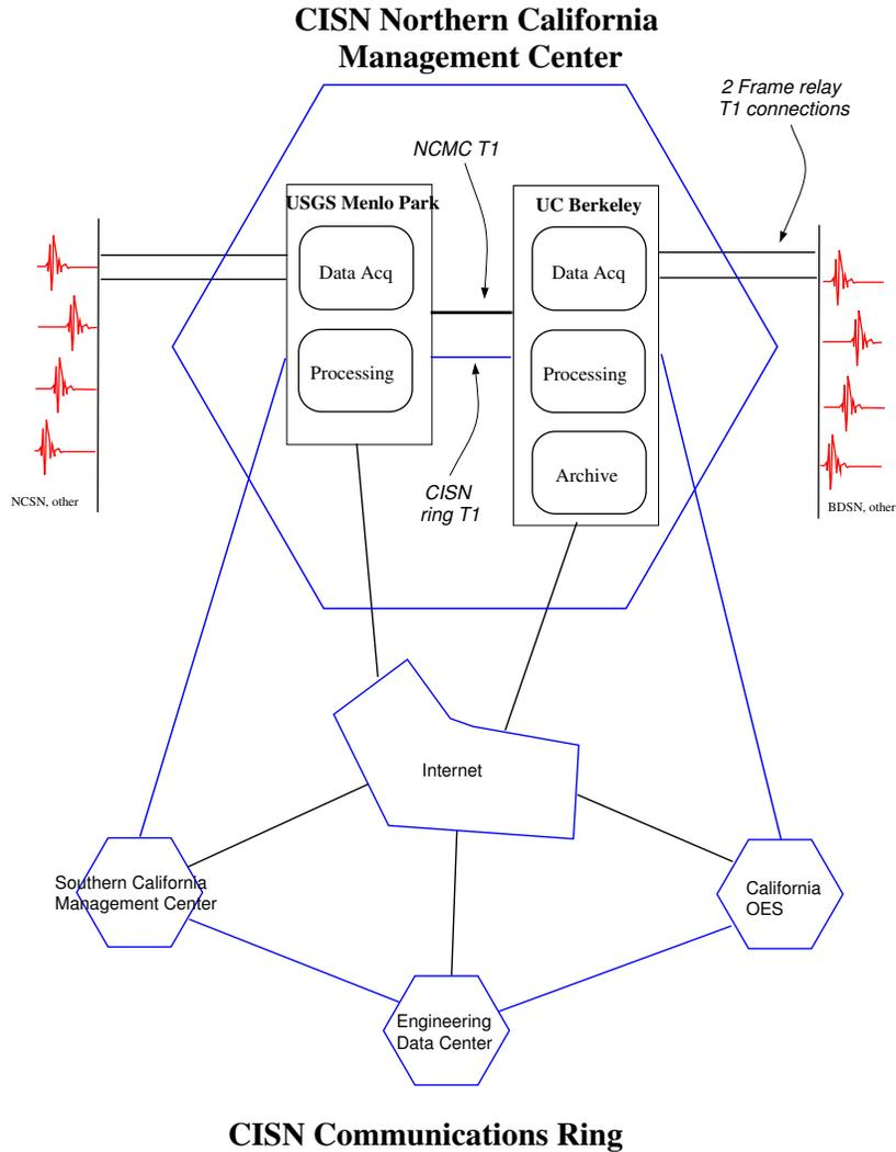
Figure 3.9: Schematic diagram illustrating the connectivity between the real-time processing systems at the USGS Menlo Park and UC Berkeley, forming the northern California Management Center, and with other elements of the CISN.
