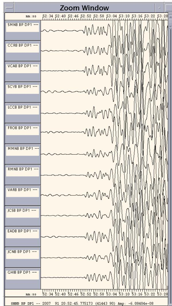
Figure 3.13: Plot of P-wave seismograms of the  $M_w$  8.1 Solomon Islands earthquake of April 1, 2007 20:39:56 (UTC) (9892 km S54E of Parkfield, CA; depth 10 km) recorded on the DP1 (vertical) channels of the 13 HRSN borehole stations. Here vertical component geophone data have been deconvolved to absolute ground velocity, 0.5-5 Hz, BP filtered. All the P waveforms have the same first motions and their subsequent arrivals are highly similar.
