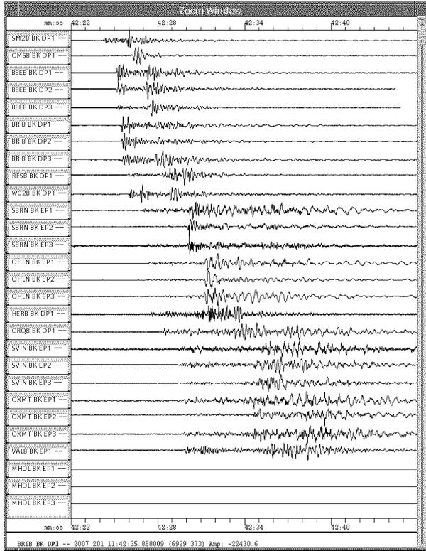
Figure 3.11: Plot of unfiltered P-wave seismograms, recorded on the geophones of the 14 operational NHFN borehole stations for a recent Bay Area earthquake (20 July 2007, M4.2 Piedmont, CA). The stations have been ordered by increasing distance from the event (top to bottom). It is immediately apparent from this simple display that station MHDL was dead and needed immediate attention.
