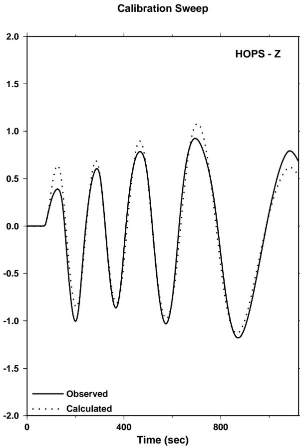
Figure 3.29: Plot of the HOPS STS-1 vertical seismometer observed time series response (solid line) and the corresponding theoretical time series response (dashed line). The best fitting theoretical response was determined via an adaptive migrating grid search to find the  $T_s$  and  $h_s$  which maximizes the variance reduction. The best fit was obtained for  $T_s = 360.08$  seconds and  $h_s = 0.6768$  critical.
