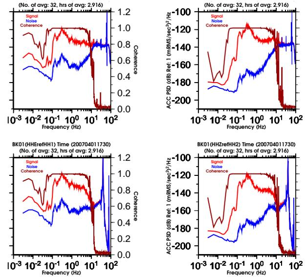
Figure 3.28: Results for the STS-1's in the presence of background noise. The traces are the same as in Figure 3.27. The lower and upper frequencies at which the coherence degrades from near unity varies among the sensors. Coherence bandwidth is a measure of the performance of the sensors.
