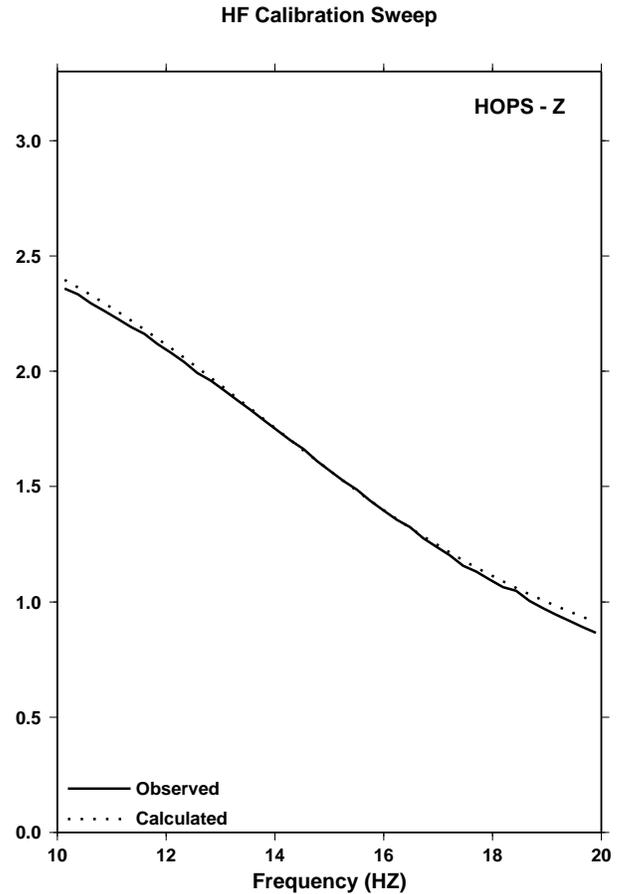
Figure 3.30: Plot of the HOPS STS-1 vertical seismometer observed phase response (solid line) and the corresponding theoretical phase response (dashed line). The best fitting theoretical response was determined via an adaptive migrating grid search to find the  $f_g$  and  $h_g$  which maximizes the variance reduction. The best fit was obtained for  $f_g = 14.998$  Hz and  $h_g = 0.371$  critical.
