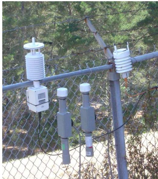
Figure 3.26: Cluster of MET sensors under test at BRIB. The sensors from left to right are; Paroscientific; BSL MET 2, BSL MET 1, and Vaisala. The electronics for the BSL MET sensors are remotely located approximately 40 feet away in the vault which contains the BRIB supporting hardware.
