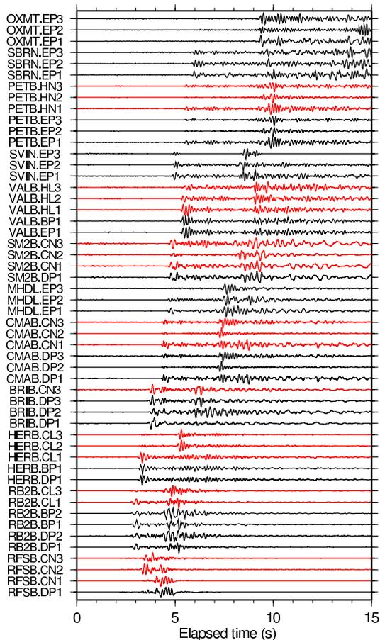
Figure 3.14: Plot of ground accelerations recorded on the geophones (black traces) and accelerometers (red/gray traces) of the 12 NHFN borehole stations in operation at the time of a recent Bay Area earthquake (5 March 2012,  $M_w$  4.0 near El Cerrito, CA). The traces are filtered with a 1-8 Hz bandpass filter, scaled by their maximum values, and ordered from bottom to top by distance from the epicenter.
