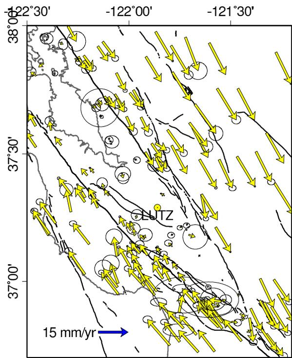
Figure 3.22: Velocities from BAVU3 $\beta$ , including BARD stations, as well as campaign and PBO stations. Yearly velocities are relative to station LUTZ, marked by a yellow circle.
