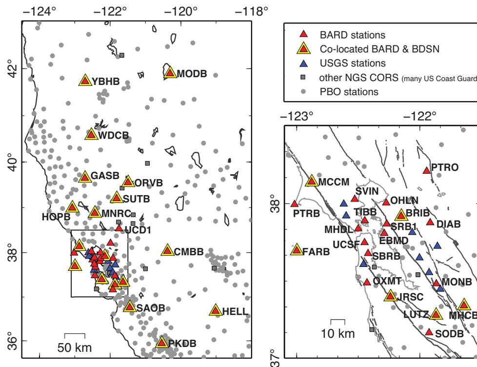
Figure 3.21: Map of the BARD Backbone network and surrounding PBO sites in Northern California. Box in left figure indicates the extent of the figure on right.
