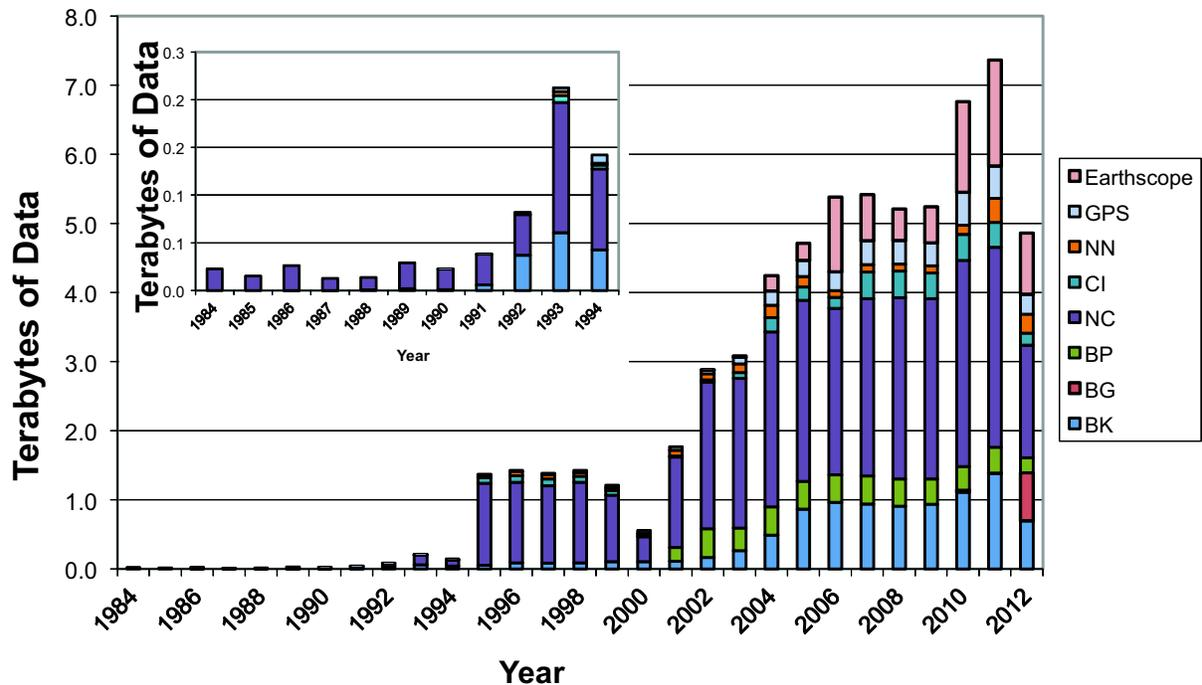
Figure 3.25: Figure showing the total volume of data archived at the NCEDC, broken down by data year.
