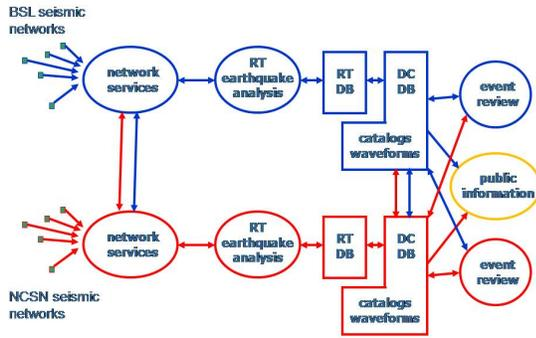
Figure 3.29: Details of the new Northern California processing system, which has been operational since mid-June, 2009. Network services processing, that is, production of picks, ground motion amplitudes, and other reduced information, occurs at both datacenters, and the information is exchanged. Complete earthquake information processing systems exist on both sides of the San Francisco Bay, and up-to-date information is exchanged by database replication.
