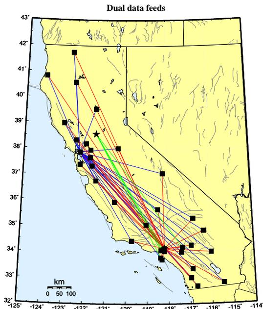
Figure 3.10: Map showing the original 30 stations selected to send data directly to the Northern and Southern California processing centers, and the 5 stations that send data directly to the Engineering Data Center and the Southern California processing center. Due to reductions in funding, now data from only 10 SC stations arrive directly at UCB and data from 12 UCB stations are sent to Caltech.
