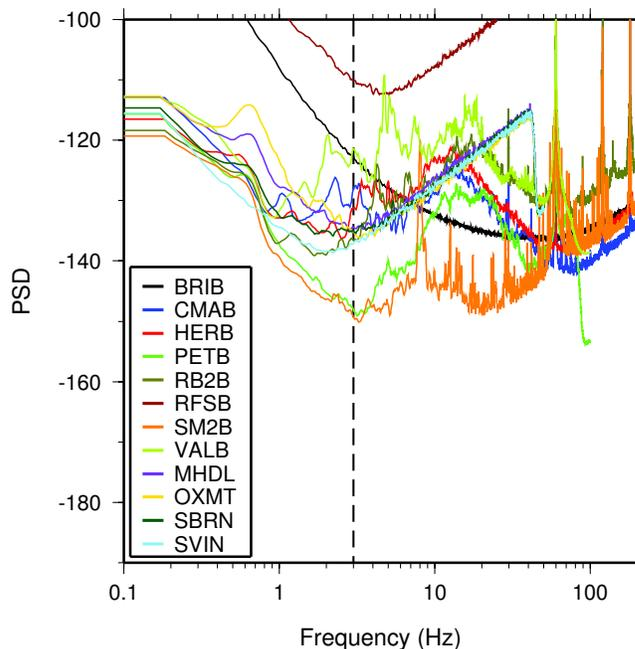
Figure 3.13: Plot showing typically observed background noise PSD for the vertical DP1/EP1 channels of the NHFN borehole stations as a function of frequency. The data are for a 1000 sec period on January 1, 2012 beginning at 01:00 (AM) local time. The PSD ranking (lowest to highest) of the non-mPBO stations (top panel) in operation at the time given at 3 Hz (near minimum PSD for most NHFN stations) is:
