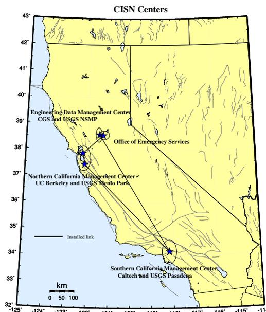
Figure 3.9: Map showing the geographical distribution of the CISN partners and centers. The communications “ring” is shown schematically with installed links (solid lines). It was initially a ring of dedicated T1 connections between the partners. The connections are now less robust, as reduced funding has required that the dedicated service was discontinued. Connections are now available as Internet tunnels.
