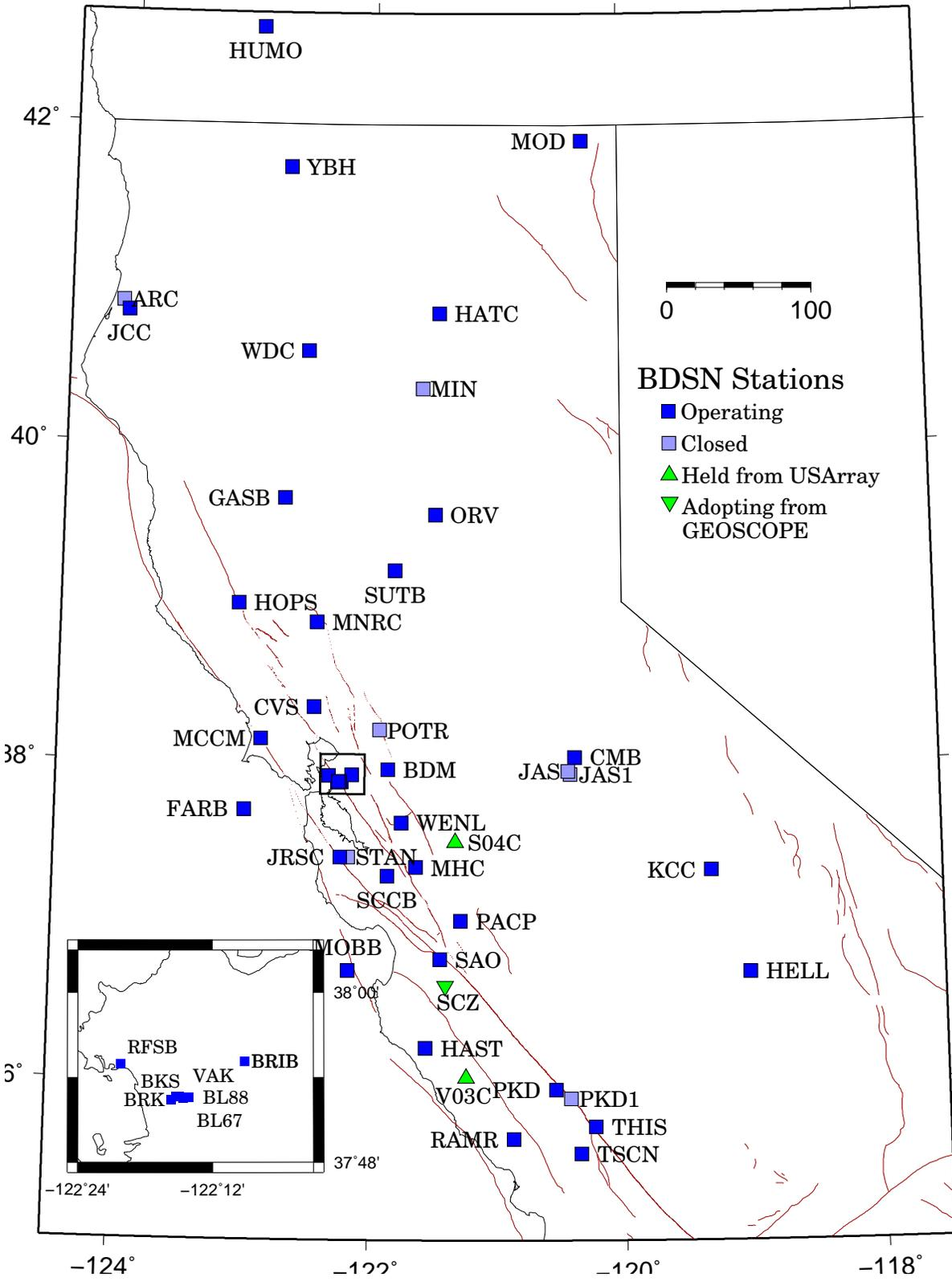
Figure 3.2: Map illustrating the distribution of BDSN stations in Northern and Central California. In the inset map, the order of the stations from left to right is: RFSB, BRIB, BKS, VAK, BL88, BL67, BKS, BRIB.
