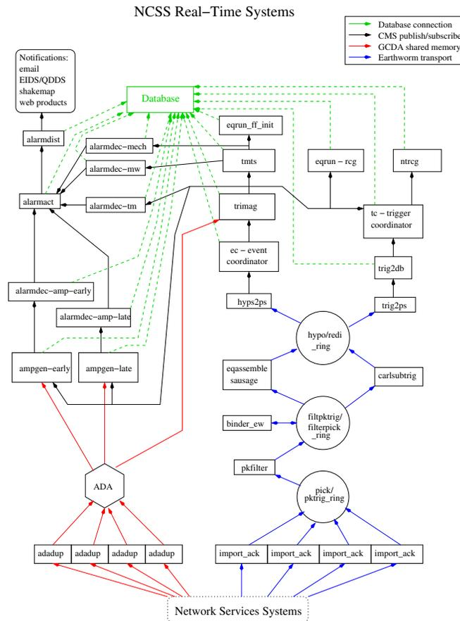
Figure 3.31: Schematic diagram of processing in the NCSS system. The design combines elements of the Earthworm, TriNet, and REDI systems
