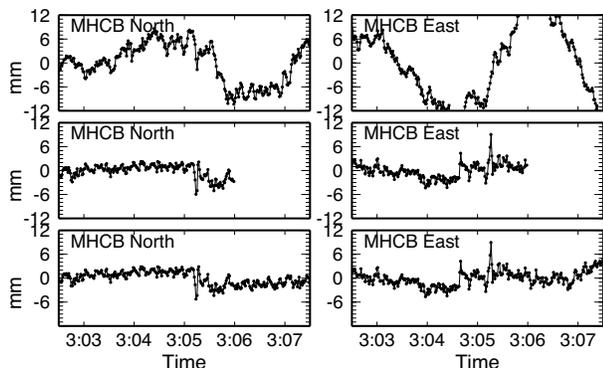
Figure 3.23: Time series of East and North motions for station MHCB during the M5.5 Alum Rock earthquake. The top row is simulated real-time data processing, the middle row is post-processing including up to a minute of data after the event origin time and the bottom row includes 10 minutes of post-earthquake data. Note that the plots are in GPS time, such that the earthquake origin time would plot as 3:05:09.
