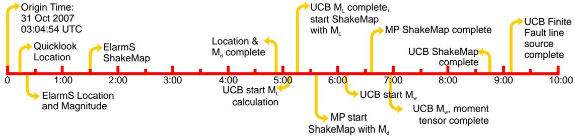
Figure 3.30: Illustration of the earthquake products timeline for the  $M_w$  5.4 Alum Rock earthquake of October 30, 2007. Note that all processing was complete within 10 minutes of the origin time.
