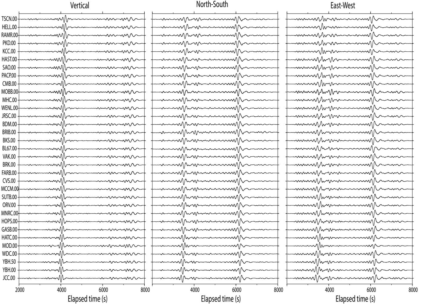
Figure 3.4: Long period (100-333 s period) waveforms recorded across BDSN from the  $M_w$  8.6 teleseism which occurred on April 11, 2012, off the west coast of northern Sumatra at 2.311 N, 93.063 E. The traces are deconvolved to ground velocity, scaled by their maximum values, and ordered from bottom to top by distance from the epicenter. The highly similar waveforms recorded across the BDSN provide evidence that the broadband sensors are operating within their nominal specifications.
