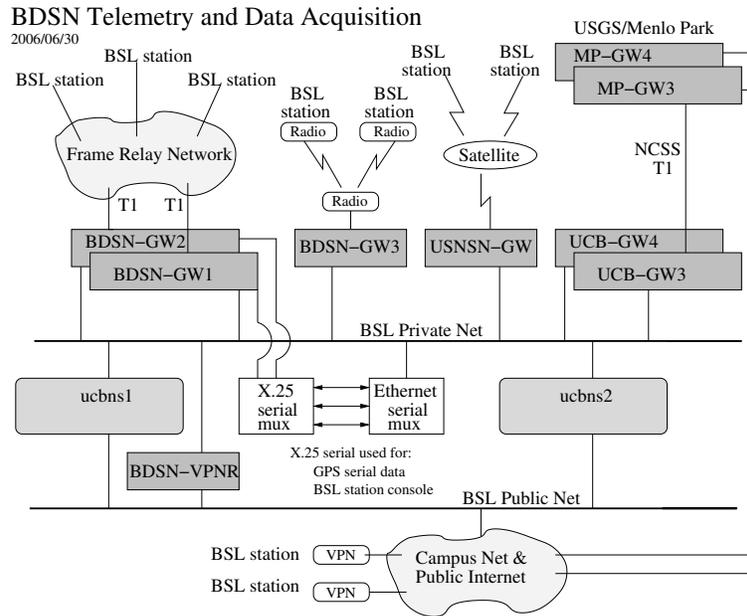
Figure 3.26: Data flow from the BDSN, NHFN, mPBO, HRSN, and BARD networks into the BSL central processing facility.
