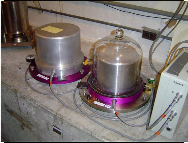
Figure 3.31: STS-1 seismometers in the Byerly Vault installed in a new pressure vessel (left) and on a warpless baseplate with a glass bell (right).
