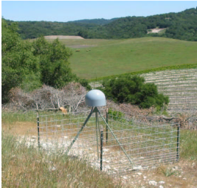
Figure R2. PBO site P526 on the Ramage Ranch. The heavy fencing around the geodetic GPS monument is required to avoid damage from grazing cattle.
