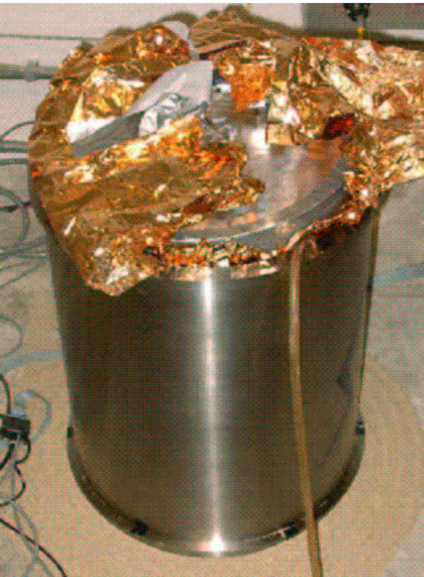
Figure 2. Titanium pressure vessel being purged with dry argon gas. Visible are the hose used to purge the air from the pressure vessel and top part of the Mylar insulation which, along with a 2 inch thick urethane foam disk, is used to insulate the top of the seismometer. By insulating the top and side of the cylindrical pressure vessel, but not the bottom, the ~2.2 Watt power dissipation of the sensor produces a stable stratification of the argon gas in the pressure vessel and inhibits the convective air currents which were generating a high background noise PSD on the CMG-1T vertical component as shown in Figure 3.
