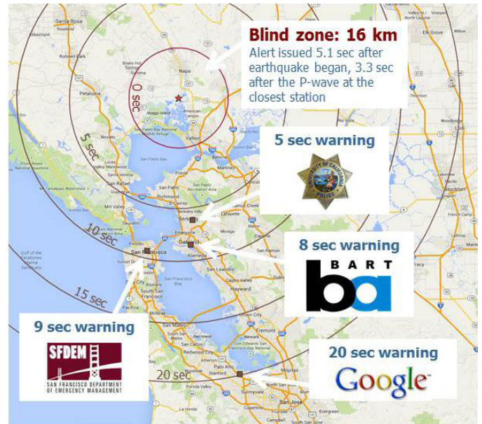
Figure 2.6.2 Warning times for UCB ShakeAlert partners for the M6 South Napa earthquake.
