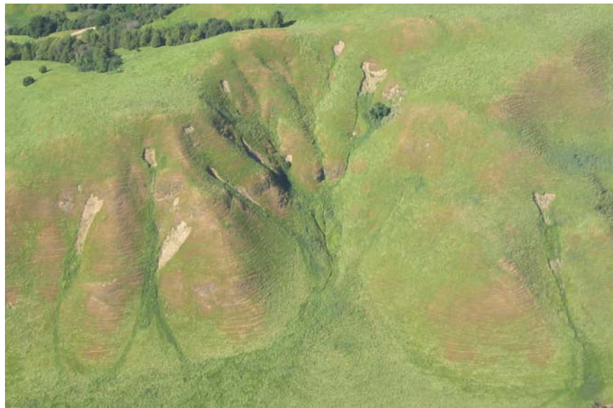
Figure 1. Shallow landslides on hillslopes near Briones, California, showing a range of size and location (note that the unvegetated scars partly include the runout portion of the slide; scene width is about 300m).
