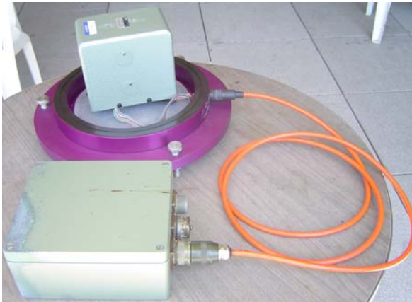
Figure 2. Photograph of an STS-1 sensor and its electronics. At the top is the mechanical sensor placed on a baseplate surface (the standard environmental shielding is not shown). Below is the electronics module. The sensor cable (orange) is attached to the “Sensor” connector on the electronics and a to hermetic feedthrough on the baseplate. The “Monitor” and “Remote” connectors (unused) are also visible on the electronics box.
