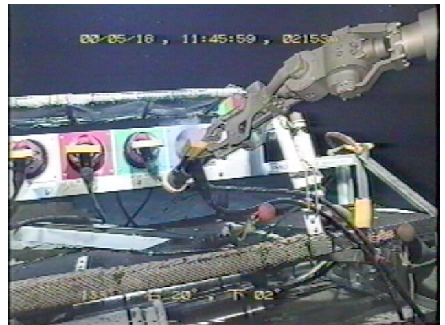
Fig. 3: Photographs of JBX and manipulator operation at the ocean-bottom
