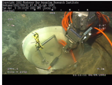
Figure 2: left: Installation of the seismometer package inside the PVC caisson. This was later completely covered by glass beads. Right: Trawl-resistant enclosure for the recording and battery packages. This snapshot was taken as the ROV Ventana was bringing the cable from the seismometer package in order to connect it onto the recording package. The first time such a remote underwater connection was attempted during the MOISE experiment, it took 2.5 hours to succeed and led to a redesign of the geometry of the instrument packages. The ROV operators are now able to do this routinely in less than 5-10mn.
