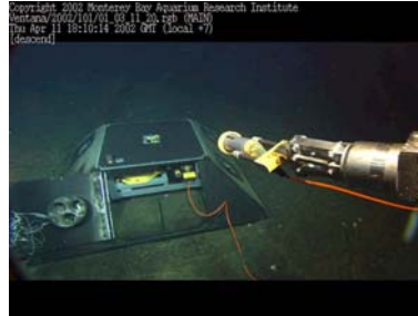
Figure 2: left: Installation of the seismometer package inside the PVC caisson. This was later completely covered by glass beads. Right: Trawl-resistant enclosure for the recording and battery packages. This snapshot was taken as the ROV Ventana was bringing the cable from the seismometer package in order to connect it onto the recording package. The first time such a remote underwater connection was attempted during the MOISE experiment, it took 2.5 hours to succeed and led to a redesign of the geometry of the instrument packages. The ROV operators are now able to do this routinely in less than 5-10mn.
