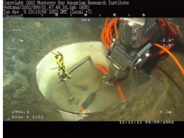
Figure 2: left: Installation of the seismometer package inside the PVC caisson. This was later completely covered by glass beads. Right: Trawl-resistant enclosure for the recording and battery packages. This snapshot was taken as the ROV Ventana was bringing the cable from the seismometer package in order to connect it onto the recording package. The first time such a remote underwater connection was attempted during the MOISE experiment, it took 2.5 hours to succeed and led to a redesign of the geometry of the instrument packages. The ROV operators are now able to do this routinely in less than 5-10mn.
