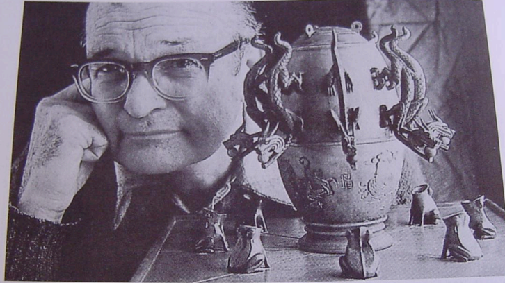
Figure 3.1 The author with model of Chang Heng's seismoscope. Balls were held in the dragons' mouths by lever devices connected to an internal pendulum. The direction of the epicenter was reputed to be indicated by the first ball released. [Photo by National Geographic Magazine.]
