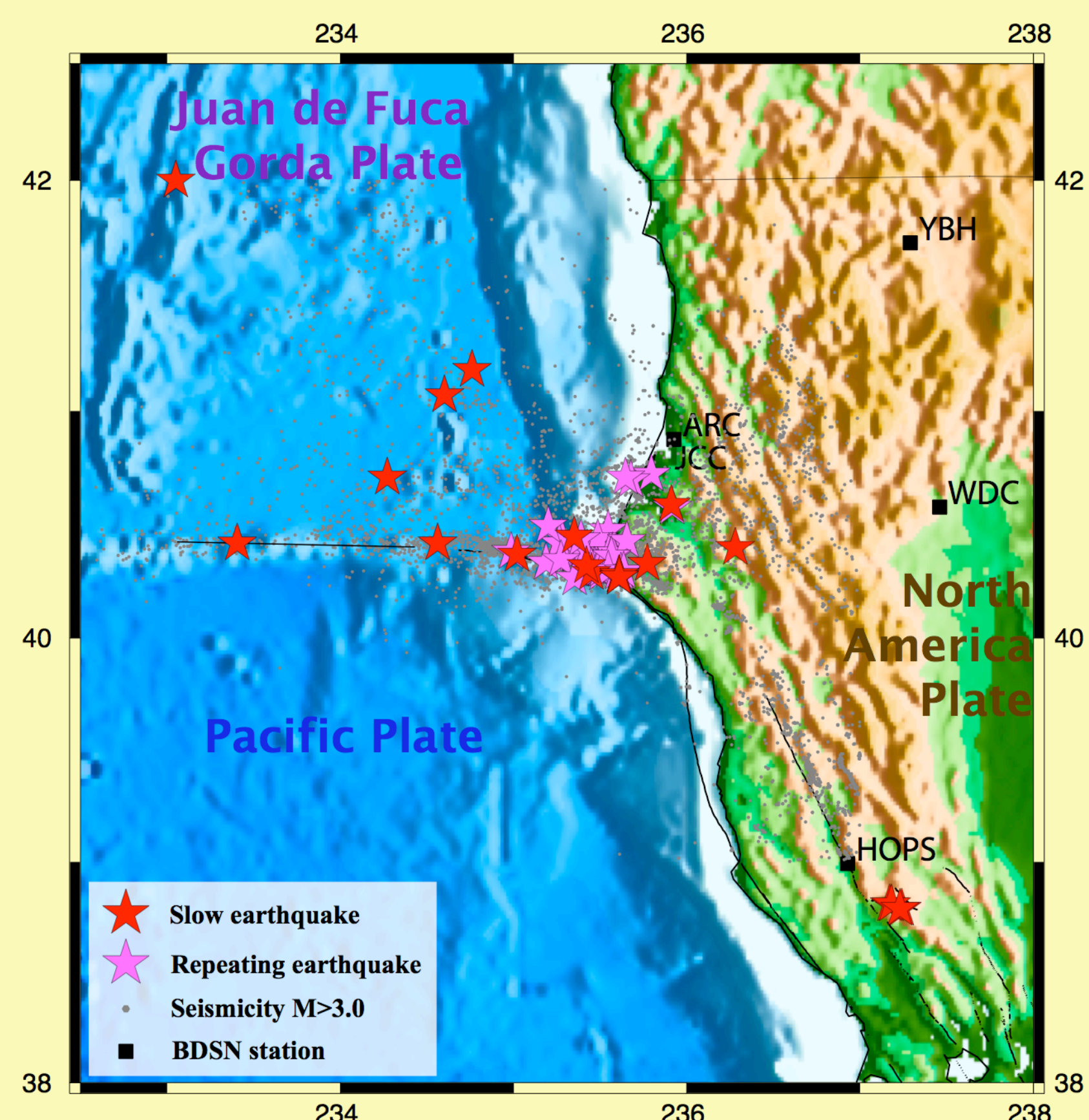
Figure 2: Map of the unusual seismicity in the Mendocino Triple Junction. The slow/low-stress-drop events are represented by the red stars, the repeating earthquakes by the pink stars, the black squares indicate the BDSN stations.
