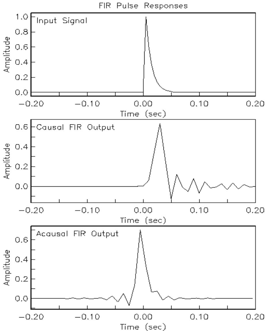
**Figure 5.** Comparison of acausal and causal FIR filter response to a common impulsive input signal (top trace).
