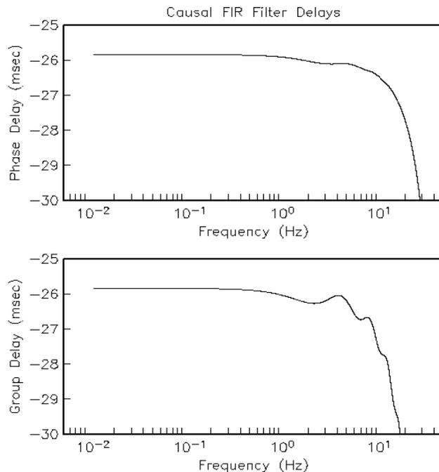
**Figure 4.** Causal divide by two FIR filter phase and group delays.
