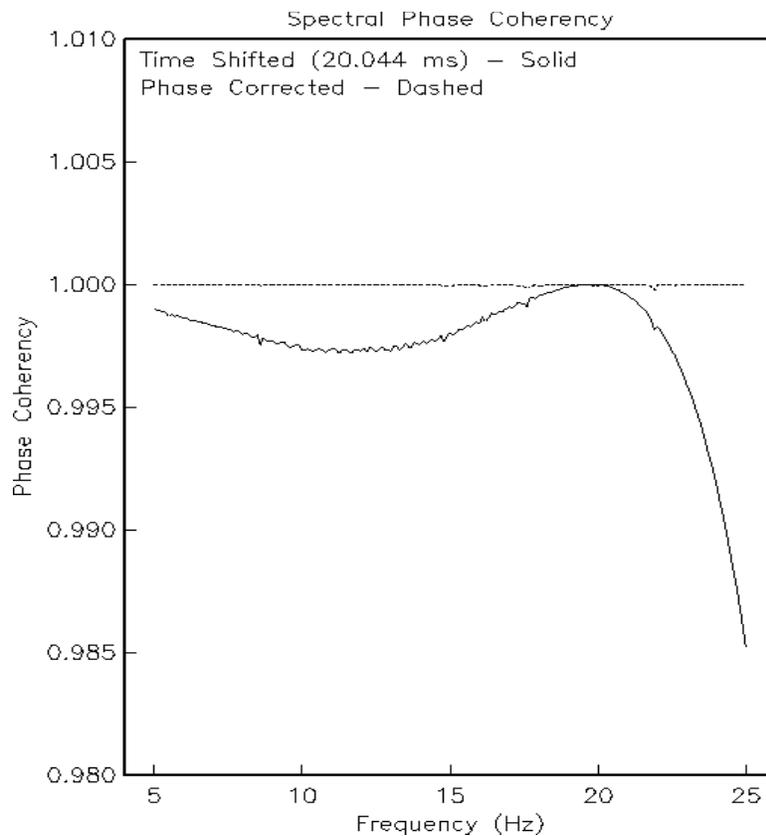
**Figure 8.** Spectral phase coherency as a function of frequency between the acausal and causal time series shown in Figure 7. The solid line is the results of determining the time shift (20.044 ms) which maximizes the spectral phase coherency in the 5-25 Hz frequency band and the dashed line is the results of the determining the spectral phase coherency after correcting for the frequency dependent phase distortion of the casual filter.
