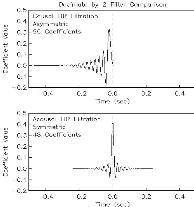
**Figure 1.** Plot of causal and acausal FIR decimate by two filter coefficients. The vertical dashed line represents the output sample time and the solid lines represent the FIR coefficients at each input sample time.
