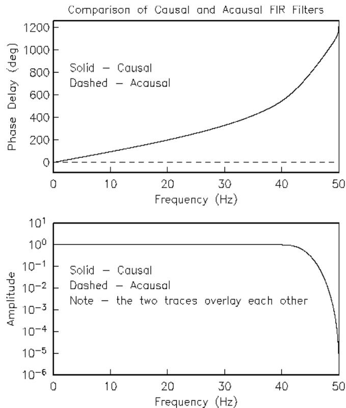
**Figure 2.** Spectral amplitude and phase response of acausal and causal divide by two FIR filters.
